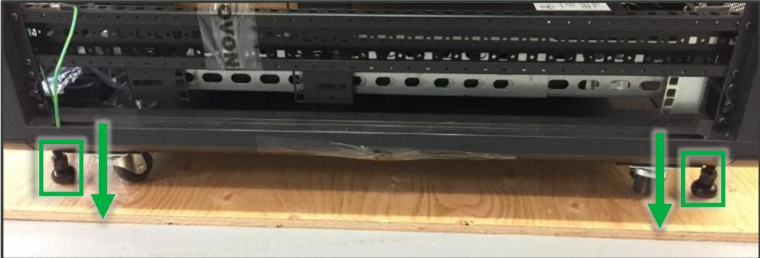
Once the rack is in its final position, lower the leveling feet to bear the full weight of the rack.
