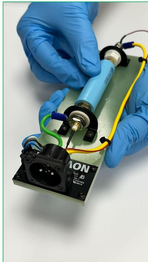
**Note:** After inserting the cell holder, if the voltage and temperature readings do not appear, apply slight pressure to the rear of the cell holder to ensure individual voltage and temperature contacts are mated properly.
