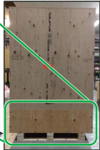
Locate the four (4) leveling feet at the base of the rack. Using a 3/4" wrench, adjust their height until the rack is sitting on them, lifted clear of the wooden shipping bracket
